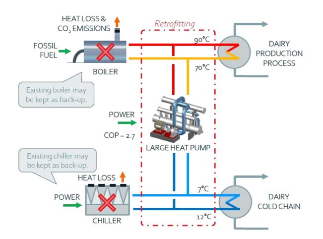
Large heat pump can be applied in food & beverage sector providing simultaneously cooling and heating services. This H/C solution maximizes heat pump technology' benefits, thus saving both heat losses from conventional refrigerated water chillers and fossil fuel for heat generation.
