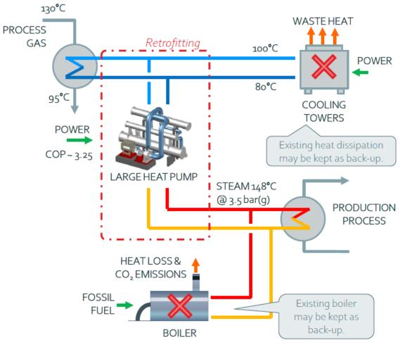
Large heat pump can be applied in the refinery sector to provide widely used steam via heat recovery from available waste heat sources. There are many potential applications for heat pump technology; here only one of them is presented.
