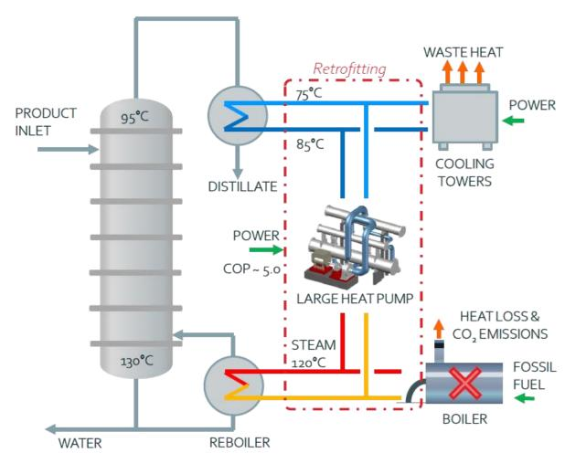
Large heat pump can be applied in the chemical sector to provide widely used steam via heat recovery from available waste heat sources. There are many potential applications for heat pump technology; here only one of them is presented.
